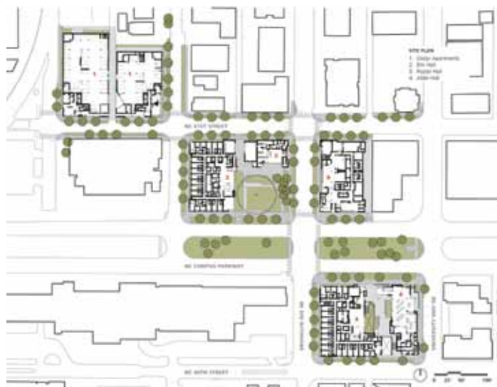
The first of four planned phases, the new UW campus project includes five buildings, each with five stories of wood-frame construction over a concrete podium.
