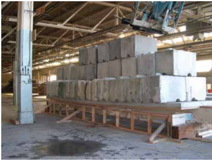
Beam #3 test just prior to failure.
