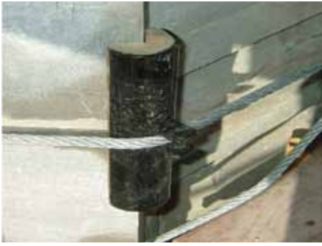
Figure 8: Corner protection for cable on stone.
