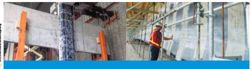
The Tyfo® Fibrwrap® systems are an innovative concept that was originally tested and validated at the structures lab in UC San Diego. With continuous testing, we invent and improve our systems worldwide. Our latest full-scale testing at UCSD has verified our patent pending anchor detailing which provides shear enhancement to columns and connections having access to only three sides.
