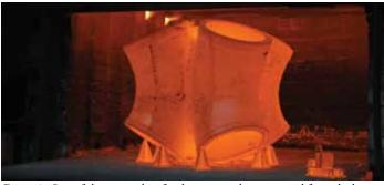
Figure 8: One of the cast nodes after having just been removed from the heat treatment oven. Courtesy of Bradken Inc.
