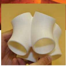
Figure 4: Rapid prototype of the cast steel node at 1:20 scale. Courtesy of Cast ConneX Corporation.
