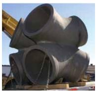
Figure 9: One of the nodes ready to ship to the machine shop. Courtesy of Bradken Inc.
