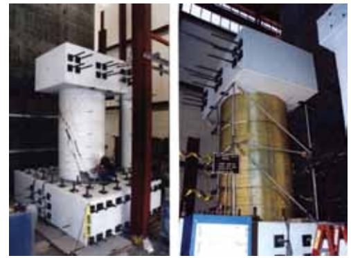
Figure 1. Testing and repair of a full-scale bridge column.
