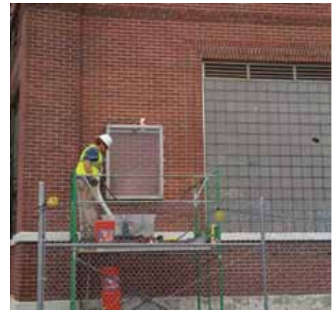
Figure 5: Moisture penetration testing for masonry walls using ASTM C1601 water chamber.
