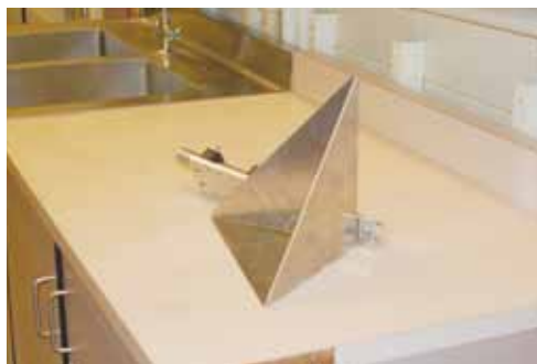
Figure 2: Ideal radar reflector.
