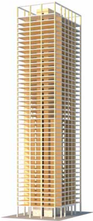
Architectural detail of the wood structure proposed in the Timber Tower Research Report.
