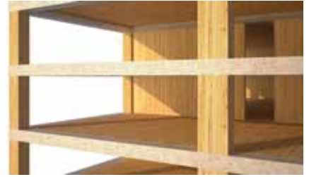
SOM's Timber Tower Research Project proposes a “Concrete Jointed Timber Frame” system that relies primarily on mass timber for the main structural elements, with supplementary reinforced concrete at the connecting points.
