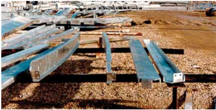
Special designs can minimize distortion when fabrications comprised of dissimilar thickness are required.
