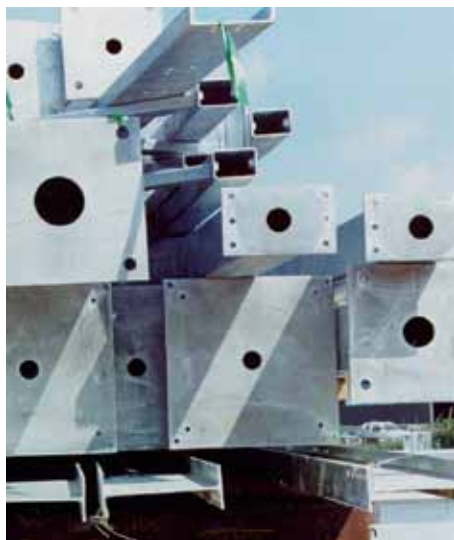
Vent and drain holes on fabricated tubing.
