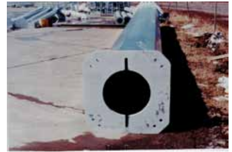
Keyhole method of draining zinc from a pole during removal from the molten zinc of the hot-dip galvanizing process.
