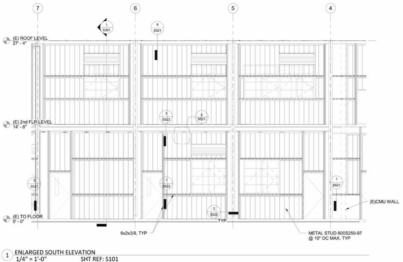
Figure 5. Typical high blast pressure wall.
