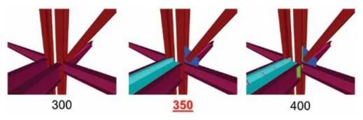
The image shows a structural steel bracing member at three LOD levels. The LOD 300 brace is for permit level structural documents. LOD 350 brace with gusset plates is for trade coordination and LOD 400 brace with welds is for shop drawings.
