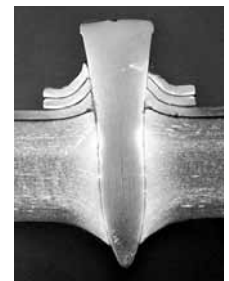
Figure 2: Robust anchorage - power-actuated fastener in steel.
