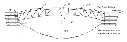
arch was the bottom chord of his truss, the upper arch was the top chord of his arch and the middle arch carried the floor to the truss. The span was almost 30% longer than his longest previous bridge.
