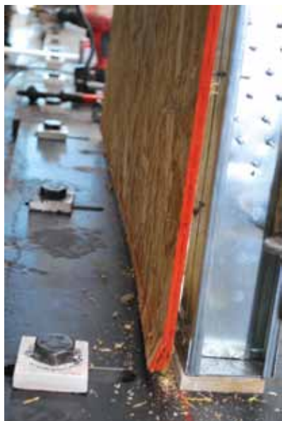
Figure 6: Non-winged self-tapping screw test assembly failure.
