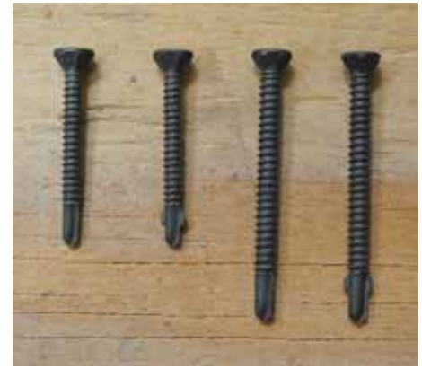
Figure 5: Winged tip and non-winged tip #8 and #10 self-drilling tapping screws.
