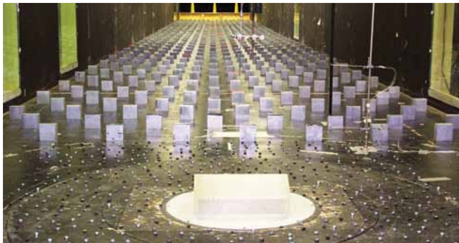
UWO wind tunnel showing model and upstream simulation of terrain roughness. Courtesy of UWO Boundary Layer Wind Tunnel.
