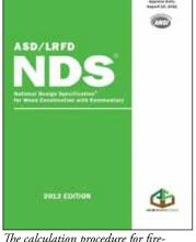
The calculation procedure for fireresistance of exposed wood members is found in Chapter 16 of AWC's National Design Specification (NDS) for Wood Construction.
