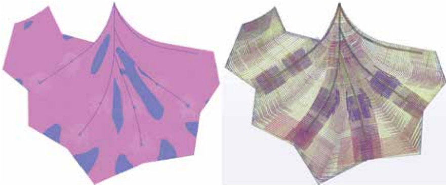
Shell stress plot on the left with areas of blue representing additional reinforcement on the Park Entrance roof. On the right, the resulting Tekla model shows all reinforcing steel. Courtesy of Pepper Construction and DNA Detailing & BIM.
