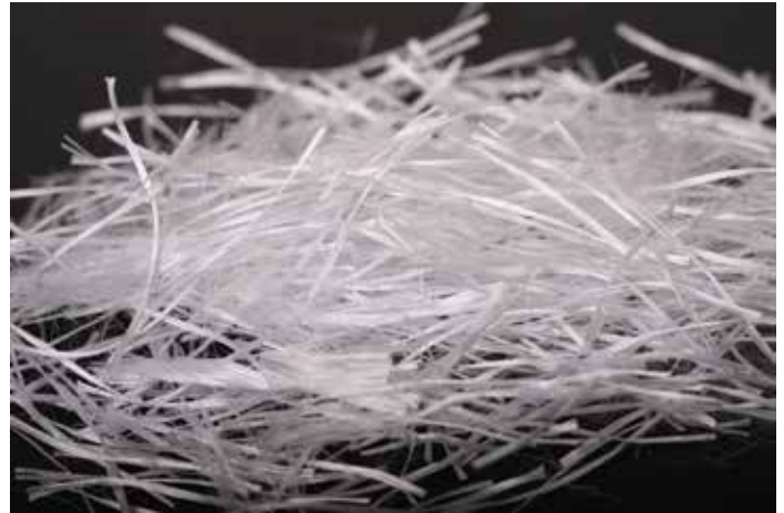
Blend of synthetic microfibrils and macrofibers for concrete applications.
