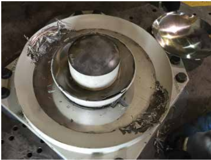
Half-size bearing with dual radius outer slider tested to extreme displacement.
