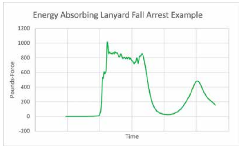
Figure 7. A force vs. time graph of an energy-absorbing lanyard arresting a test weight.
