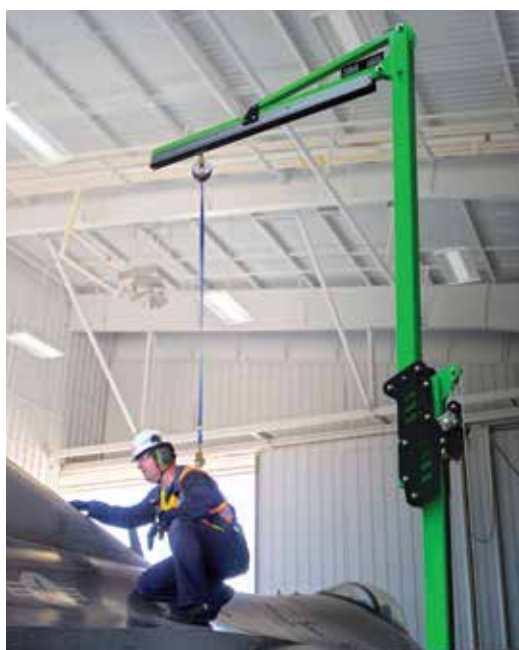
Figure 2. An Engineered Modular Jib utilized as an FPS anchorage point.
