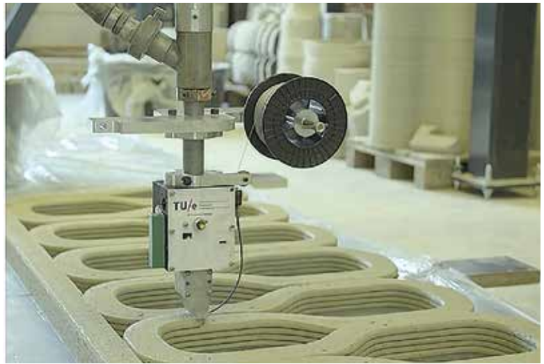
Figure 3. Integrated wire reinforcement was deposited in much the same way as the modern entrained wire printing system. Courtesy of TU/Eindhoven.
