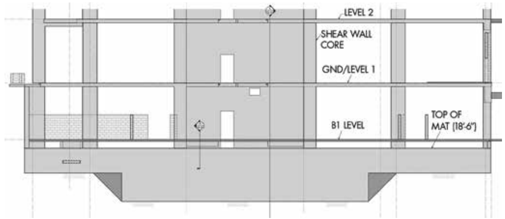
Mat foundation 7 to 15 feet thick.
