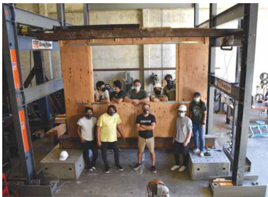
Figure 4. Full-scale experimental FTAO shear wall test specimen.
