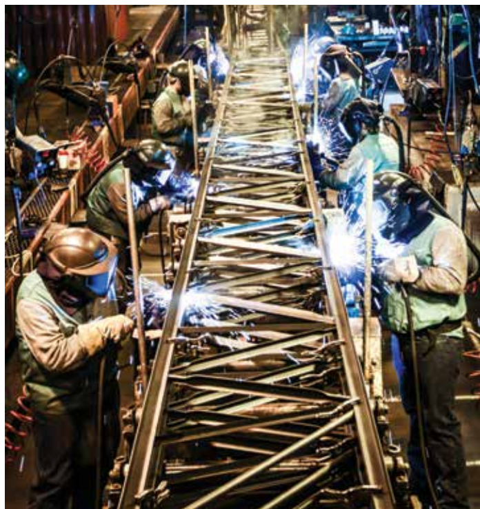
Figure 2. Welding web to chords of an open web steel joist, Vulcraft facility.
