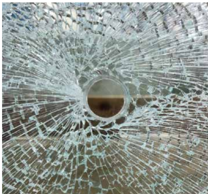
Figure 7. Testing failure at standoff hole location in a laminated glass panel.
