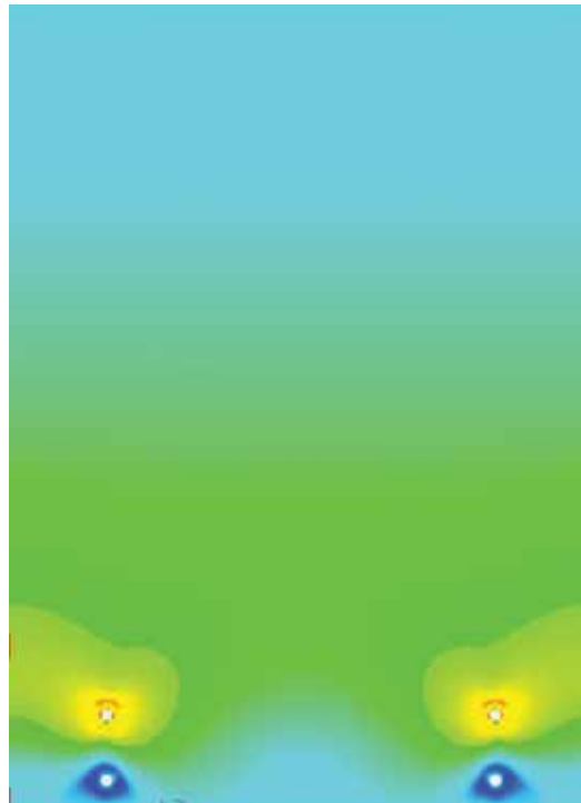
Figure 5. FEA model showing stress concentration at standoff support.
