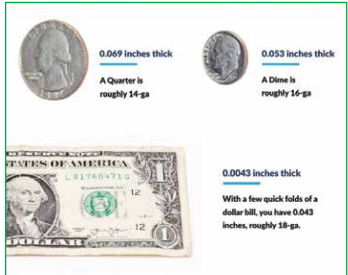
Figure 3. Common thickness reference materials.
