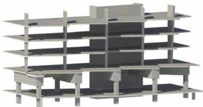
Figure 5. Tower column transfers over the garage.
