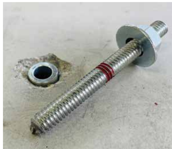
Figure 4. Due to the extreme load capacities, high-performing undercut anchors can be designed for ductile steel capacity, provided they are embedded deep enough to prevent concrete breakout.
