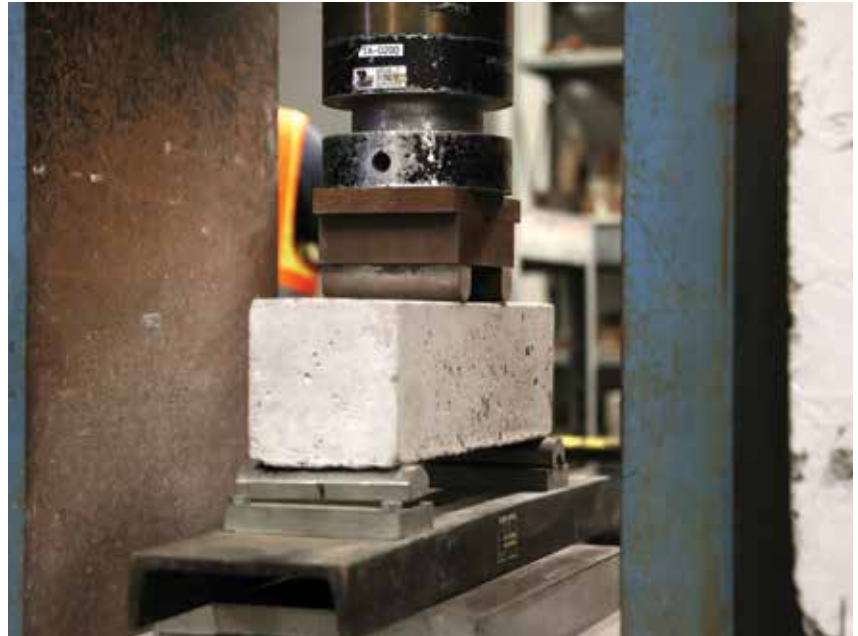
Figure 3. ASTM C78 flexural test.
