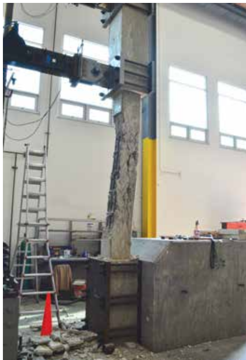
Figure 8. Shear failure in diagonal tension of the control (un-retrofitted) column and subsequent spalling of cover concrete.
