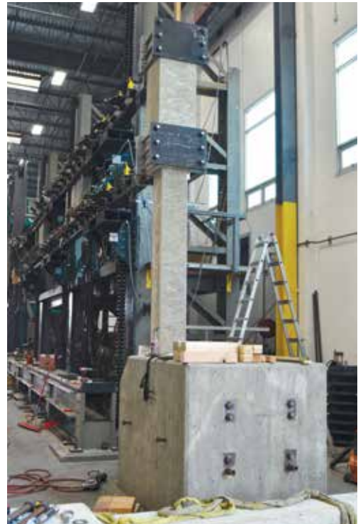
Figure 3. Control (un-retrofitted) column in the testing frame.
