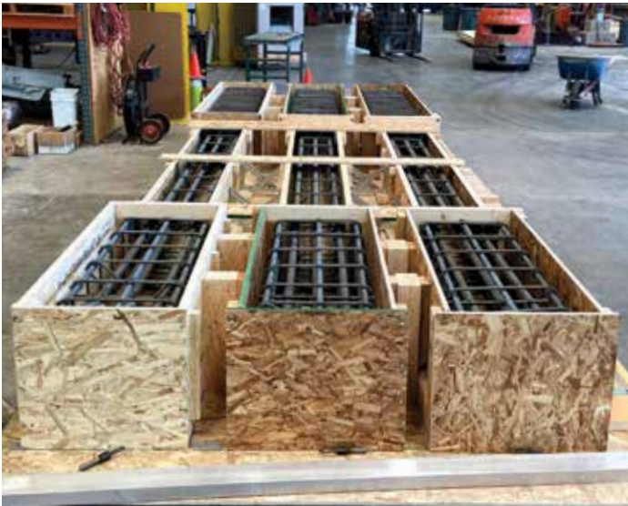
Figure 2. Column specimens during construction showing formwork and reinforcement.
