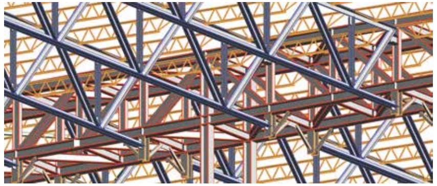
Figure 3. In a sloping cantilevered bay, the joist girders (blue) frame into the cantilever truss (red) to form the roof slope. The supporting joists (orange) slope as well.
