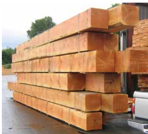
Figure 4. New timbers that have been bundled after visual grading.
