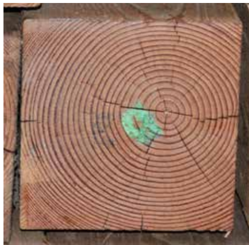
Figure 3a. Boxed heart timber with checks radiating from the pith, some that extend to the exposed faces of the timber.
