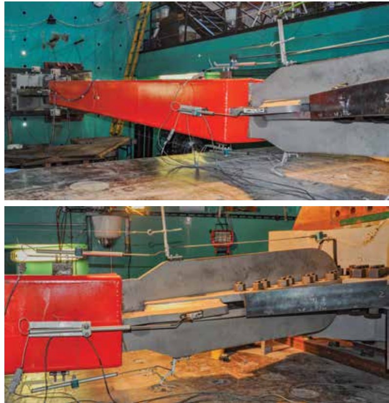
Figure 1. Global out-of-plane buckling of a BRB Test Specimen with views showing: plastic hinge at neck facilitated by restrainer local yielding (top); additional plastic hinge at gusset (bottom).
