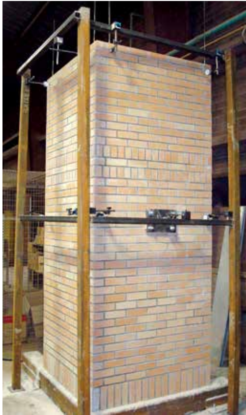
Figure 2. Corner test for warping investigation.
