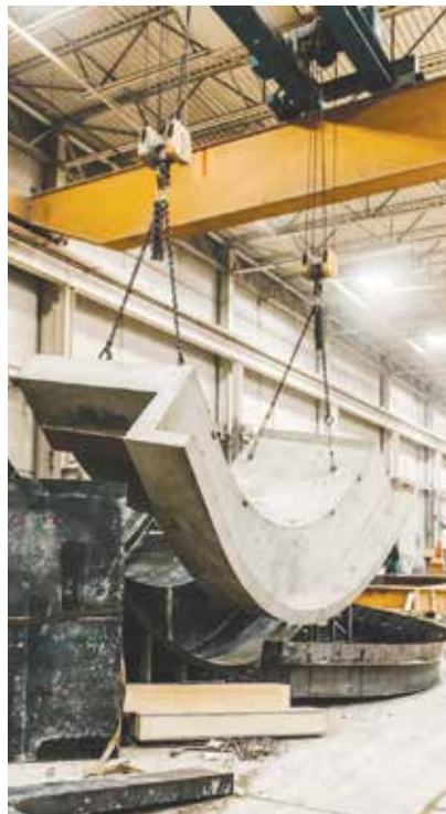
Figure 3. Complex precast radiused piece and form.
