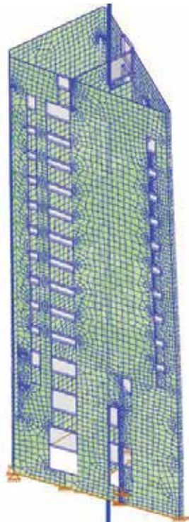
Figure 2. RISA 3D model of the core deflection.
