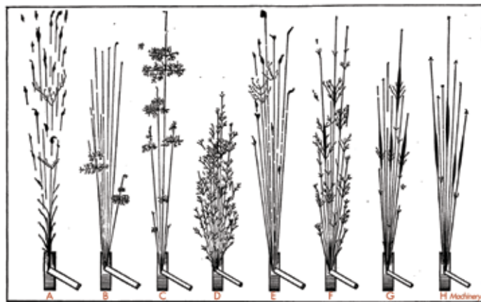
Figure 6. Diagram of sparks showing branching and forking. Part A shows wrought iron, and Parts B through E shows various irons or steels. The presence of carbon is relative to the branching or forking of the sparks. From Iron and Steel by Erik Oberg and Franklin Day Jones, 1918.
