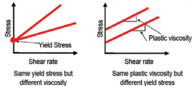
Figure 1. Drawback of slump test-predicted workability based on concrete rheology. Reprinted with permission from ACI.
