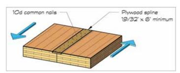
Figure 1. Longitudinal side joint.
