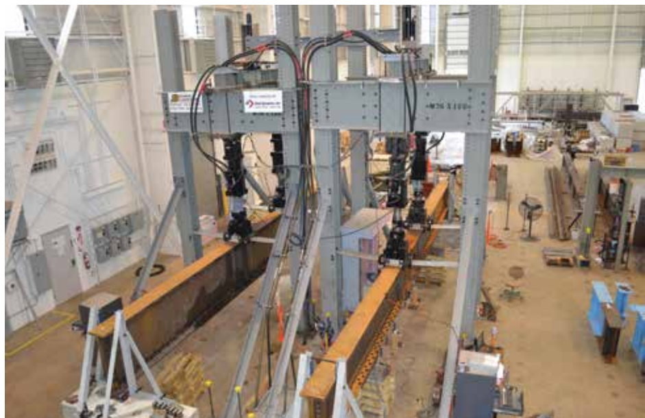
Example large-scale fatigue test of steel bridge girders (Hebdon et al., 2017).
