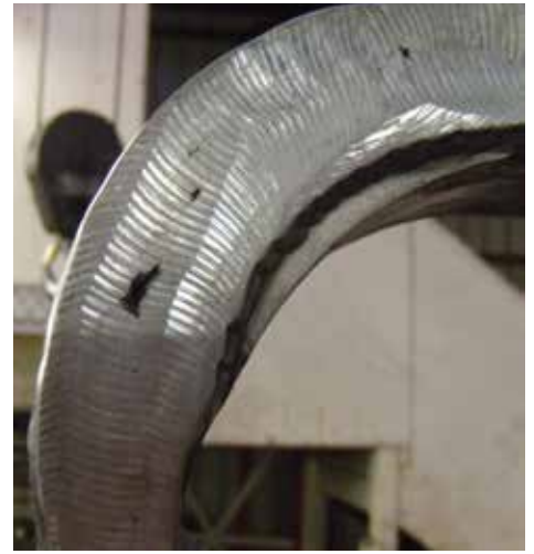
Figure 4. Machined groove weld on an AWS Code D1.2 structural aluminum weldment. The weld was rejected due to cracking and voids.
