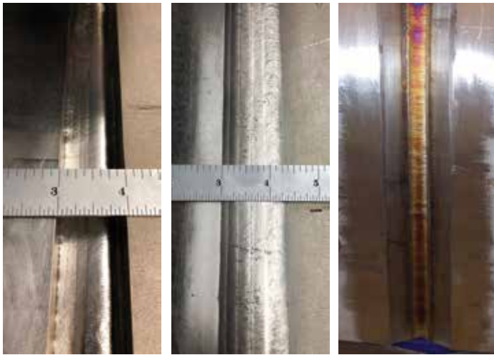
Figure 5. AWS Code D1.6 structural stainless-steel welding craftsmanship: Left and Center: Interpass and cover pass welds (mechanized GTAW) on 1.25-inch-thick plate (1G position). Right: A manual GTAW hot pass (2 nd pass) weld bead on a 1.5-inch-thick plate (3G position).
