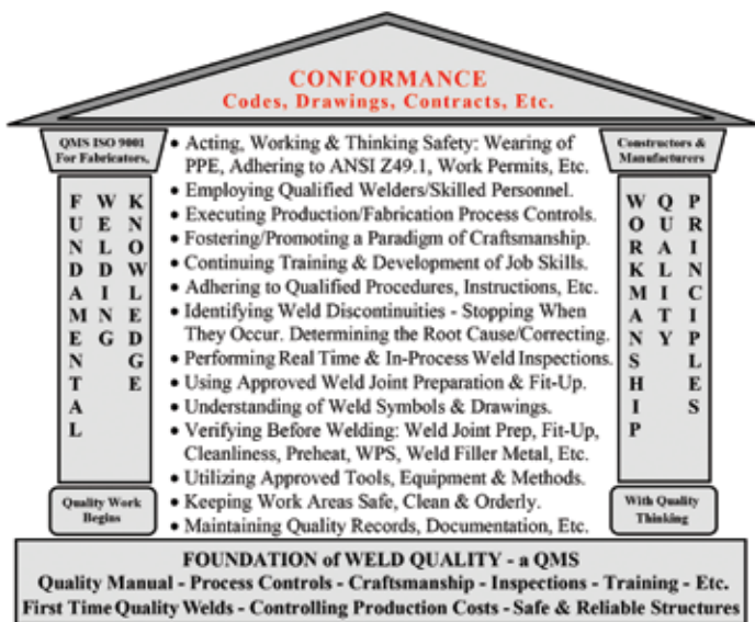
Figure 6. The House of Weld Quality symbolizes philosophies, principles, and actions essential to quality structural welding and fabrication.
