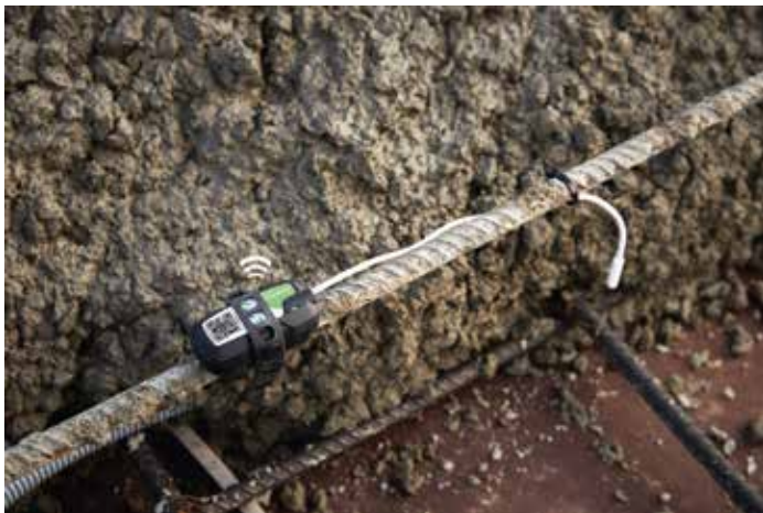
SmartRock Wireless Maturity Sensor.
