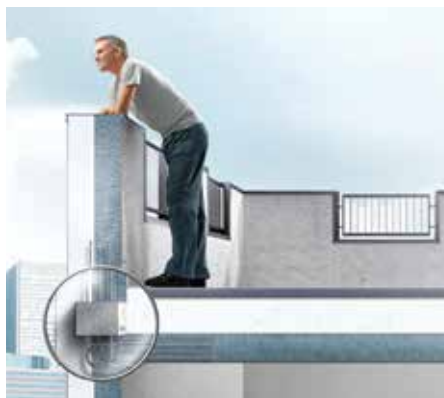
Figure 5. Rendering of a structural thermal break cast between a concrete roof slab and concrete parapet.
