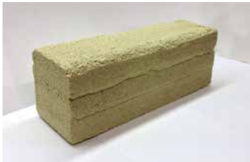
Figure 2. Enhanced articulated robot (top) and the printed sulfur concrete sample (bottom).
