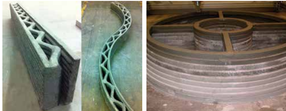
Figure 1. Layer-based construction using Contour Crafting.
