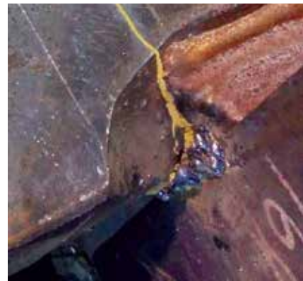
Transverse crack at the end of the weld, propagated from weld into the base metal.
