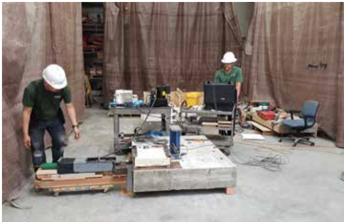
Test rig assembly shows shear loading on the helical anchor installed through the limestone panel. Courtesy of Specialized Testing Inc.
