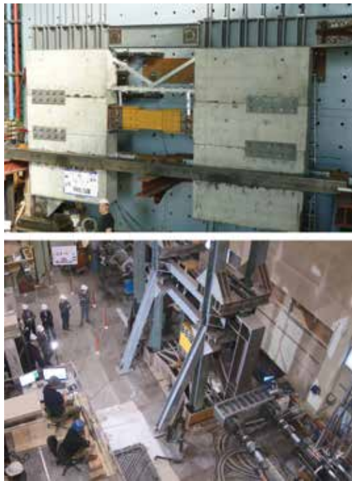
Figure 3. Full-scale uniaxial and shear racking VCD tests at the University of Toronto.
