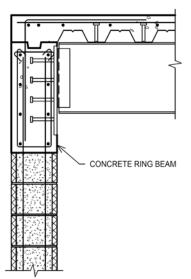
beams and concrete-topped composite metal deck has proven to be cost-effective. However, designing connections to transfer the large roof beam reactions directly into the CMU walls can become difficult. Detailing a concrete ring beam around the perimeter of the shelter roof, integral with the CMU wall, has been a successful way to facilitate more effective steel beam connections to the walls (Figure 2).
