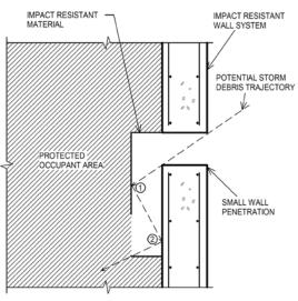
Figure 3. Baffling system example.
