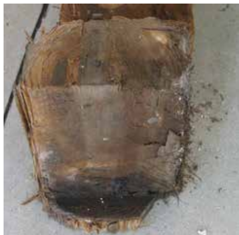
Figure 5. Left: Top of pile removed below a notch for floor beam bearing (note fuzzy wood on the right side). Right: "Fuzzy" wood and annular rings on the bottom portion of a coastal pile cut six inches below a degraded notch for floor beam. (photos are not of the same pile).
