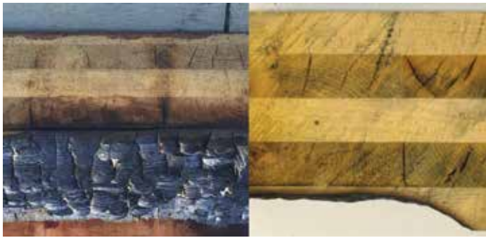
Figure 3. Left, Oblique of 5-ply CLT panel from exposed, ATF Test #3; Right, Cross-section showing char removed and remaining laminations.
